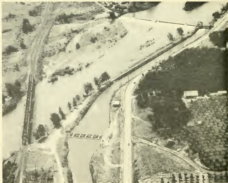
FIGURE 9.—Fish screens located in irrigation canal to stop young salmon and return them to the Yakima River.
