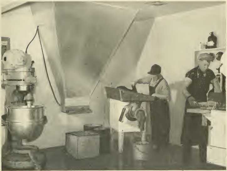
FIGURE 22.—Typical food preparation room at the Quilcene, Wash., Hatchery of the Fish and Wildlife Service. Bandsaw, grinder and vertical mixer are standard equipment. Note chutes from dry meal storage bins.
