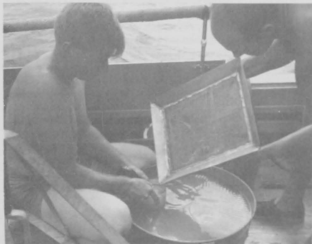
Sieving the contents of a bottom sample.
