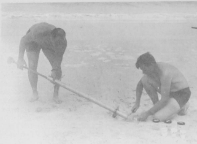
Sampling of beach sediments with a shallow-water coring device.
