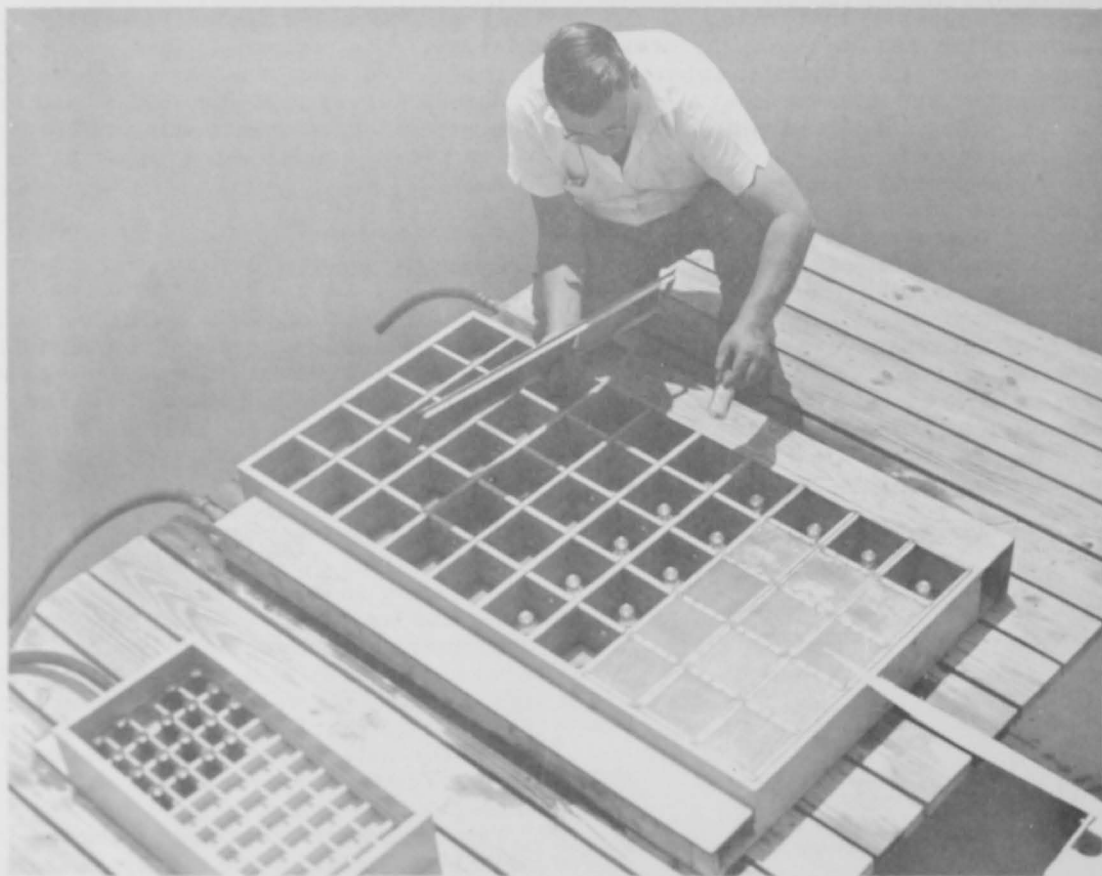
Incubator box with attenuation screens, designed for primary productivity studies in a modified version of the light- and dark-bottle method.
