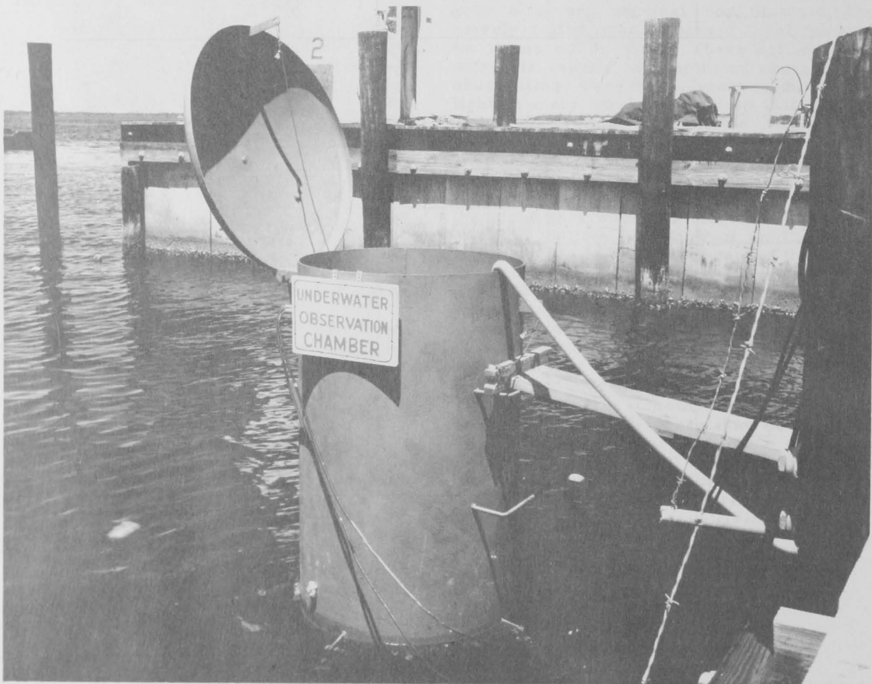
Figure 26.--Underwater observation chamber at Behavior Facility.
