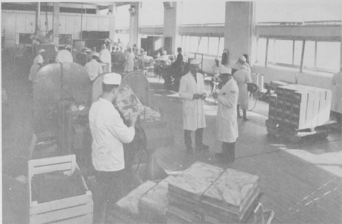
Figure 7.--Blocks of frozen fish fillets being fed into an automatic cutting machine. The blocks are cut into sticks which are then breaded and fried, Stavanger, Norway.
