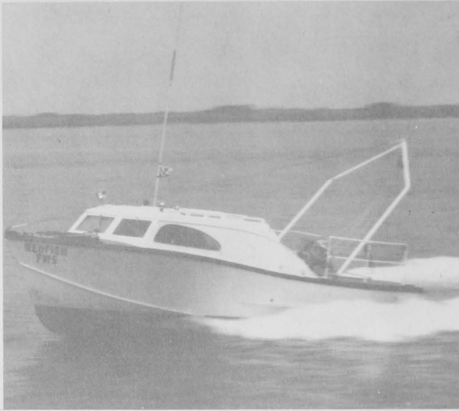
The 28-ft., tunnel-stern REDFISH, capable of operating in only 1\frac{1}{2} ft. of water and having a cruising speed of 25 m. p. h., is ideally suited for estuarine research.
