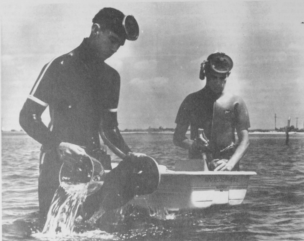
Figure 4.--Measurement of the productivity of benthic algae. One diver rinses the bell jars used to enclose the algae while the other prepares water samples for oxygen analysis.
