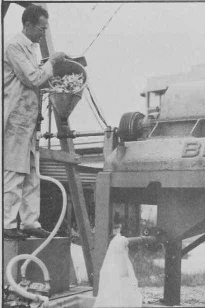
Demonstrating the separation of crab meat from shell in a horizontal centrifuge
