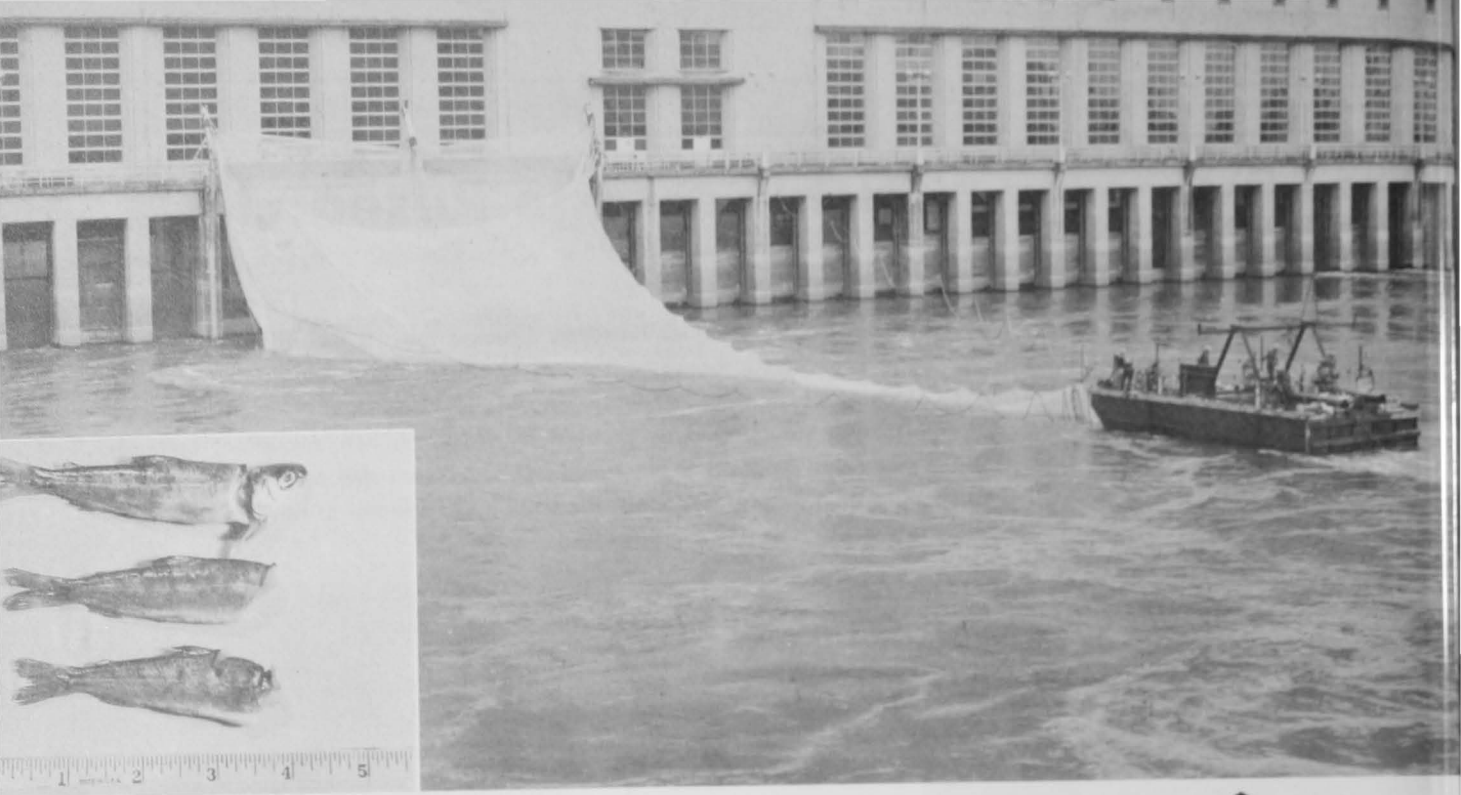
A giant net is lowered behind turbine to determine extent of damage to fingerling passing through. Insert shows sample of fish damaged by turbine.
