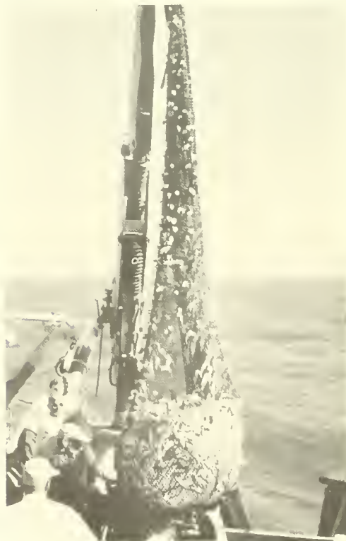
Figure 23.--Lowering the cod end of the Gulf of Mexico shrimp trawl onto the deck of the Anton Bruun after a successful haul.
