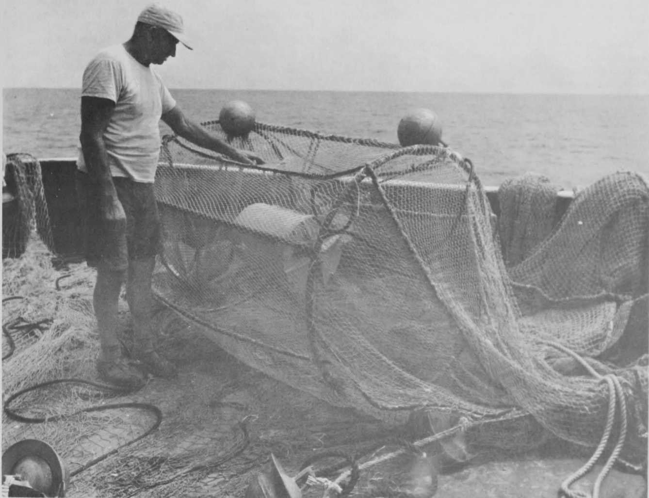
Figure 12.--Housing of underwater motion picture camera attached to its frame in the mouth of a shrimp trawl.
