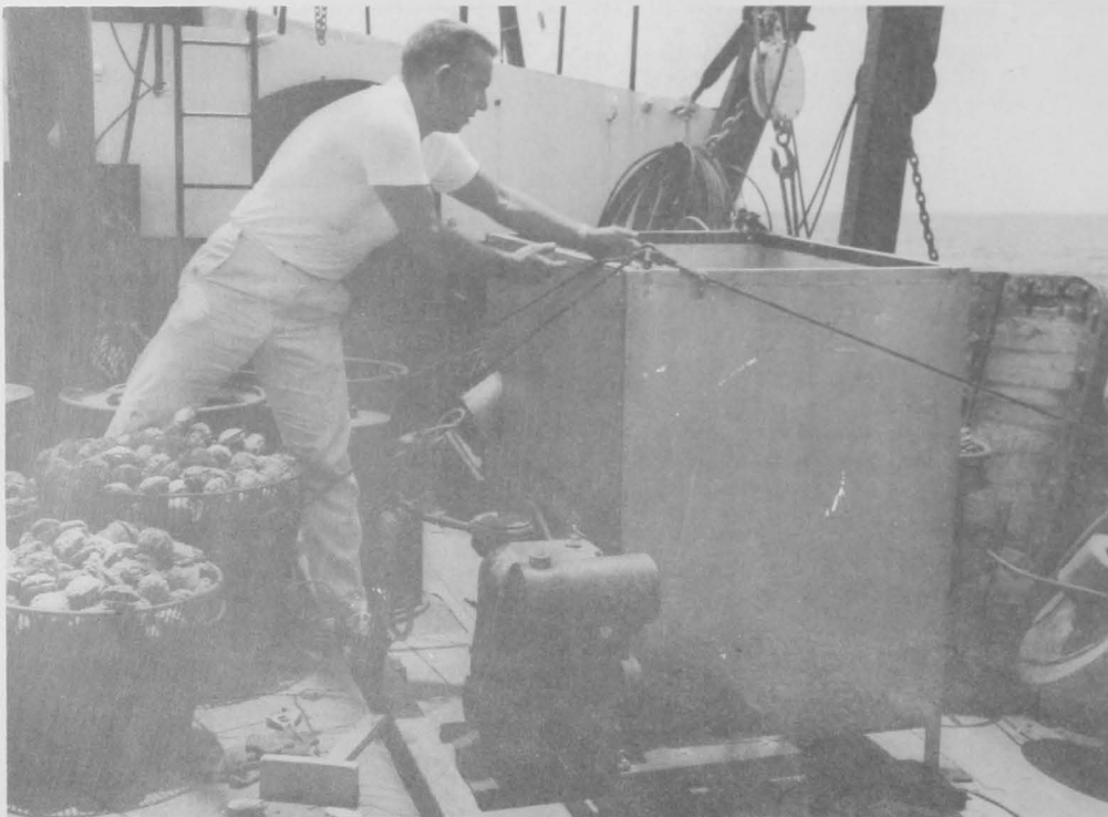
Figure 17.--Combination shucker and eviscerator. A pilot scallop shucking and eviscerating machine being tested at sea aboard the Silver Bay .
