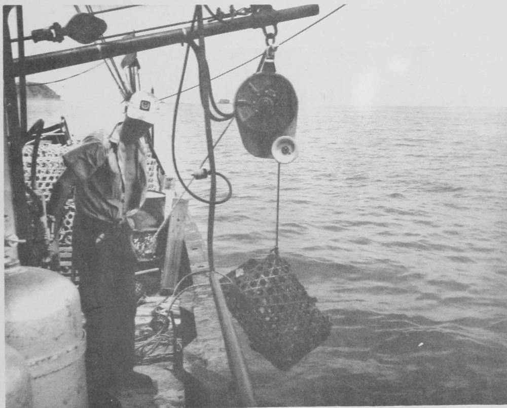
Figure 56.--After deck of Pelican showing boom and hydraulic block for hauling spiny lobster pots.
