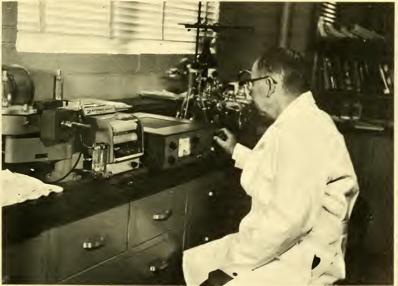
Scientific equipment in wide variety and almost fantastic capability is used in modern wildlife research. This Atomic Scanogram II Chromatogram Scanner is used at the Denver Wildlife Research Center to measure radioisotope-tagged pesticide materials on paper chromatograms. (Photo by James E. Peterson)
