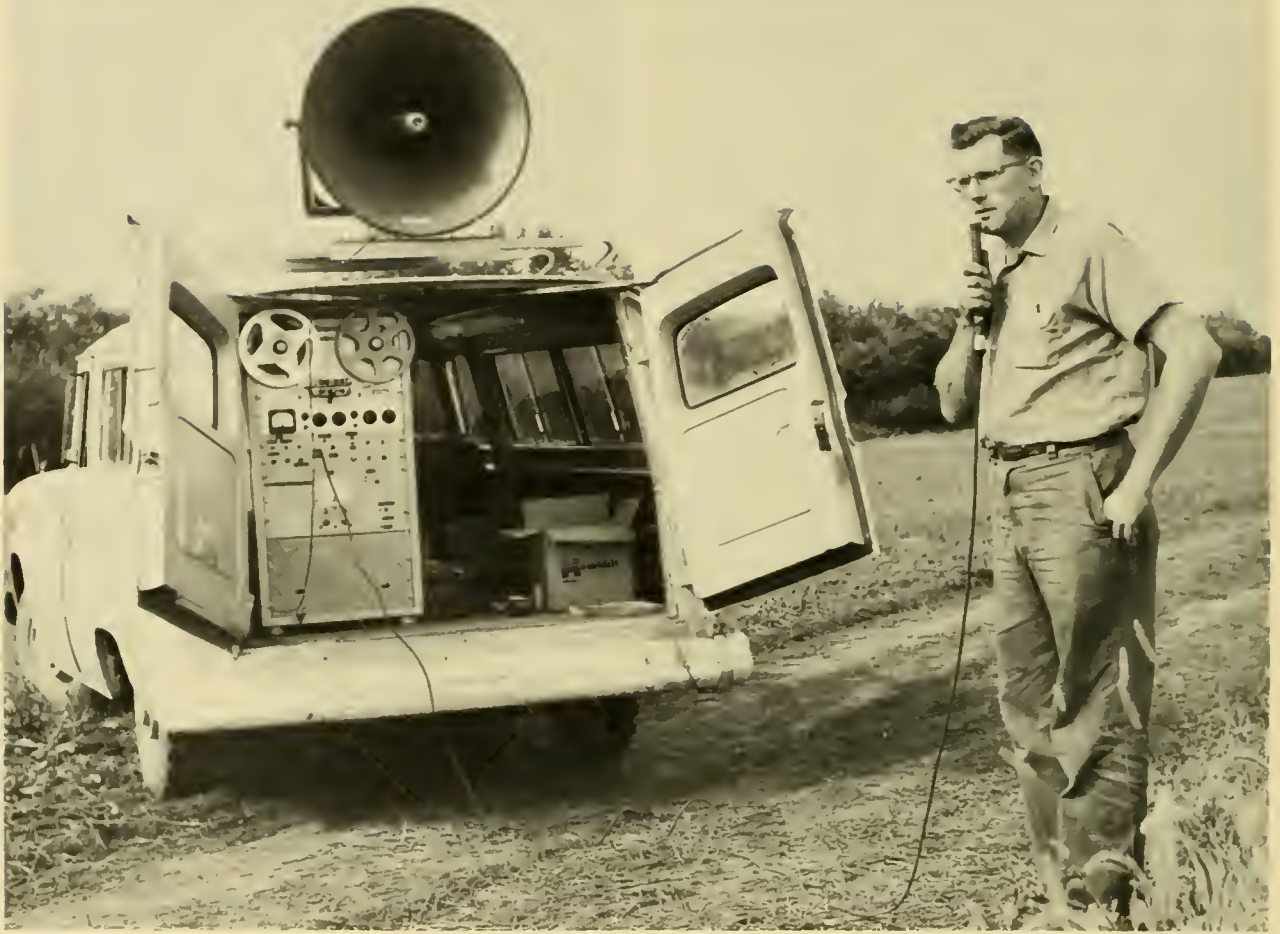
Preparation of equipment to transmit the amplified distress calls of blackbirds. This method often is effective in protecting crops from flocks of depredated birds. (Photo by Paul F. Springer)
