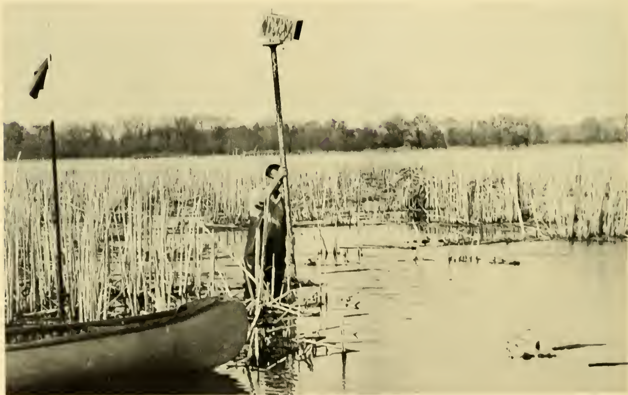
One of 60 "photographic plots" established by the New York Unit on the Montezuma National Wildlife Refuge. Automatic-sequence cameras are mounted at sampling locations to obtain a measure of duck use at different periods of the breeding and rearing seasons. The camera, in the waterproofed open-end box on the pole, is set to begin photographic surveillance of the plot at daylight the next morning, taking 1 picture every 15 minutes. (Photo by Daniel Q. Thompson)
