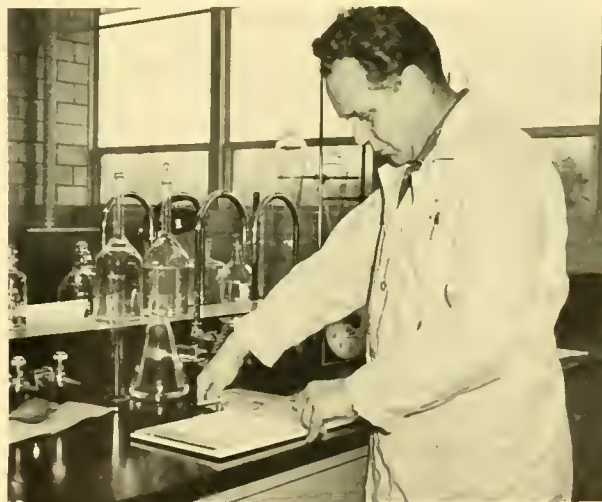
Modern and highly specialized laboratory equipment permits measurement of minutely small quantities of pesticides in animal tissues. A chemist (left) using gas chromatograph for separation and analysis of pesticide residues, and (right) a chemist preparing thin-layer chromatography plates for pesticide analysis. (Photos by Rex G. Schmidt)
