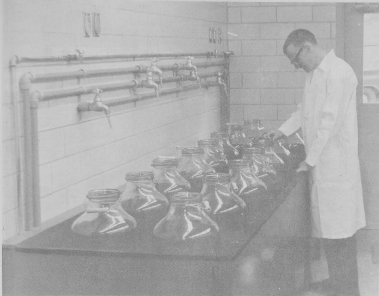
Figure 5.--View of a wet laboratory at Warm Springs showing a battery of bioassay vessels in a fiberglass tank,
