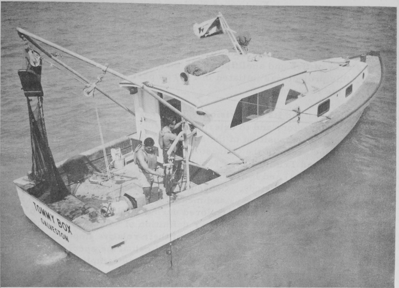
Forty-foot vessel TOMMY BOX is fitted with power equipment for sampling in deeper portions of estuarine areas.
