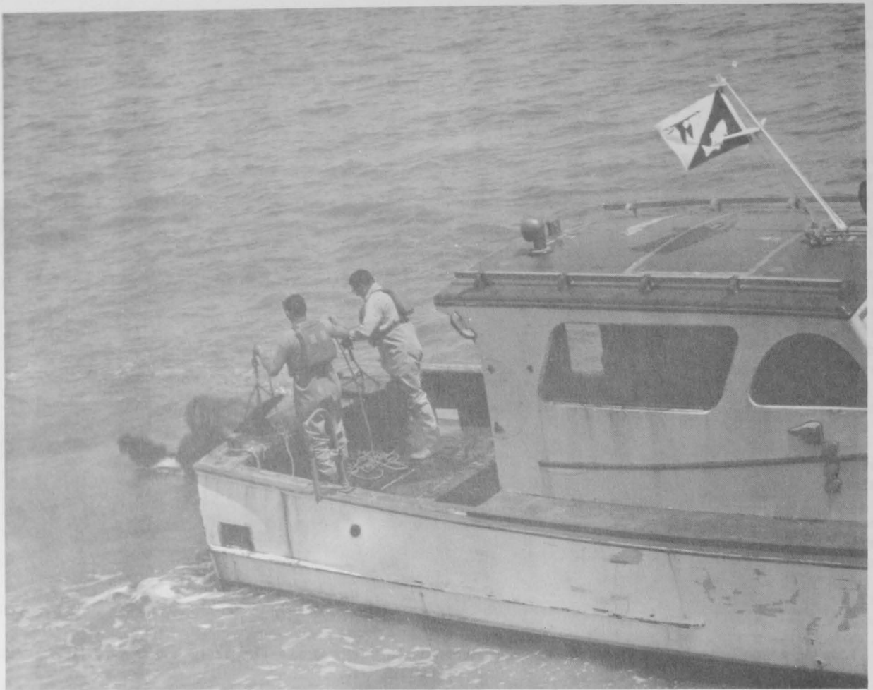
Hauling a small otter trawl aboard the Tommy Box, a 40-foot, diesel-powered boat, used by the Galveston laboratory for biological collections and hydrographic observations in the estuaries.
