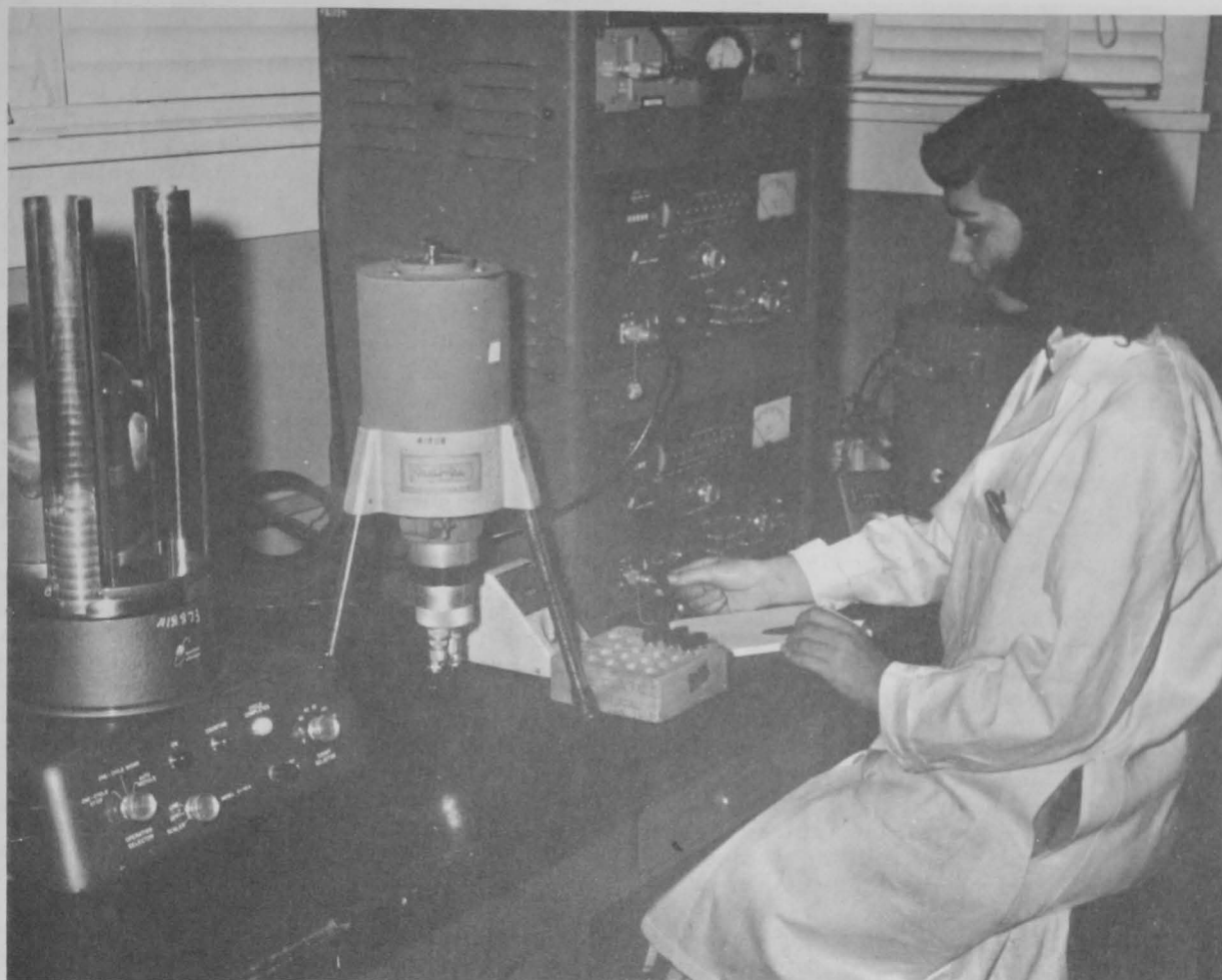
At the Bureau's Radiobiological Laboratory at Beaufort, N.C., the utilization of radioactive food by the larvae of shrimp is measured. The larvae are placed in the scintillation detector located at immediate left of control panel. Gamma rays emitted from the larvae are detected and recorded on the panel of the radioactivity counter.
