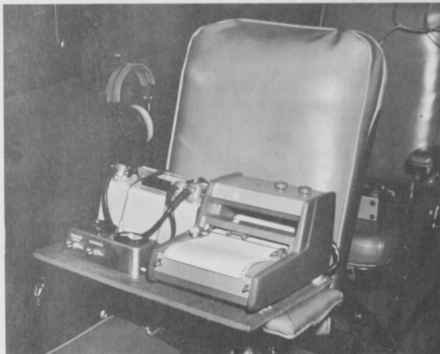
Infrared electronic console (left) and strip chart temperature recorder (right) positioned in the survey aircraft.
