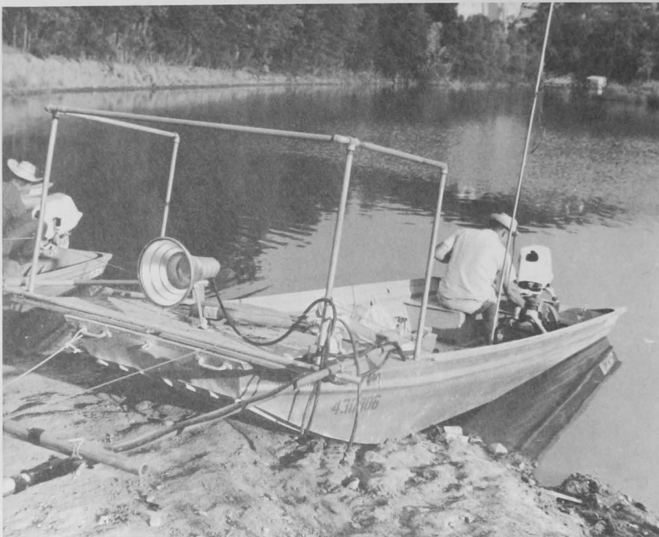
Figure 3:--One of the two similar electrofishing rigs. The one pictured uses a 230-volt A.C., three-phase generator with three flexible electrodes.
