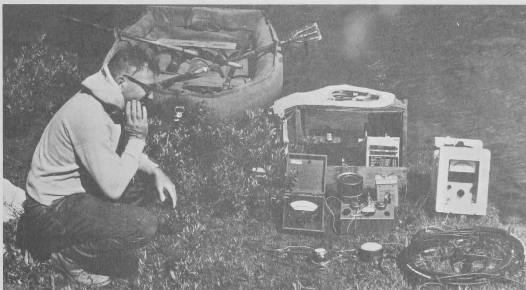
Figure 3:--Mr. Robert W. Holmes, Scripps Institution of Oceanography, contemplates photo-metric equipment used for light measurements in Lakes Edith and Cloverleaf, August 1963. Gear shown includes: deck and sea cells (selenium barrier layer), null meter, damped Rawson microammeter, collimator can for reflected light measurements, Hewlett-Packard amplifier and associated power supply (12-volt storage batteries and sine-wave inverter).
