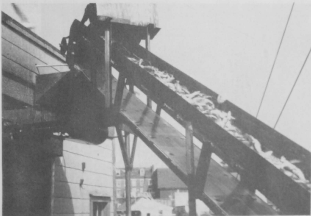
Figure 7.--Conveyor moving the whiting from the wharf to the plant.
