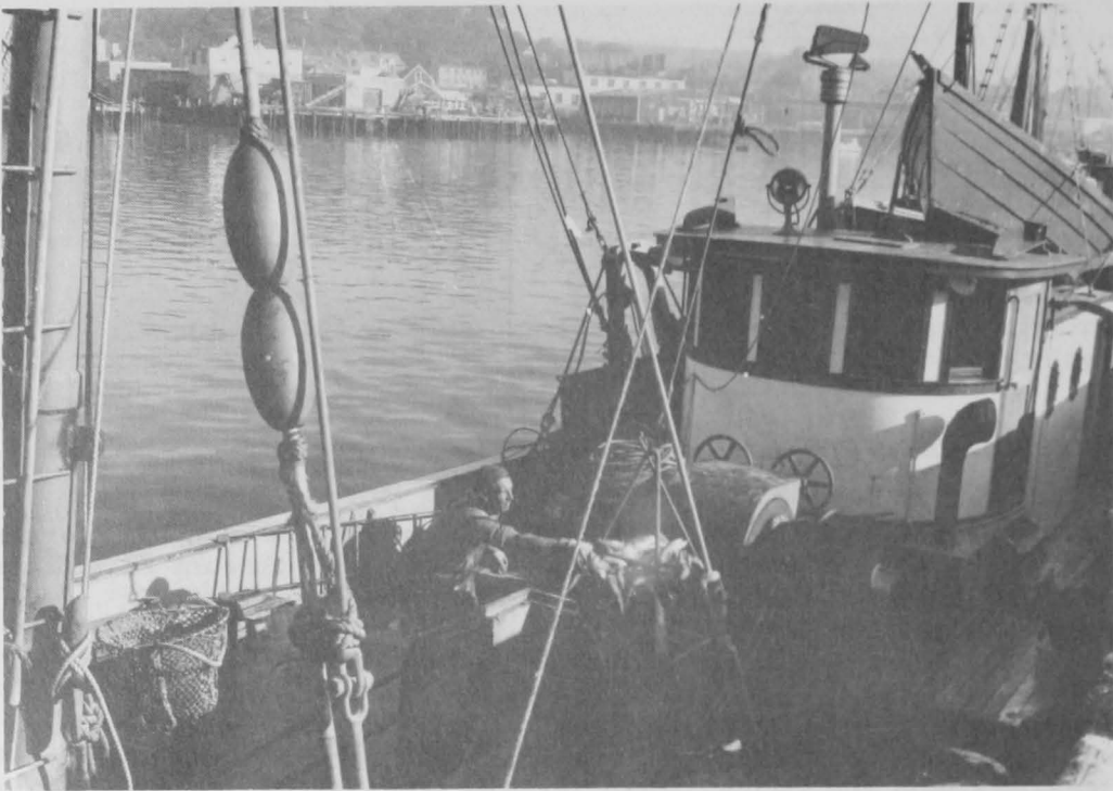
Figure 4.--Unloading a whiting vessel by means of baskets and a hoist.
