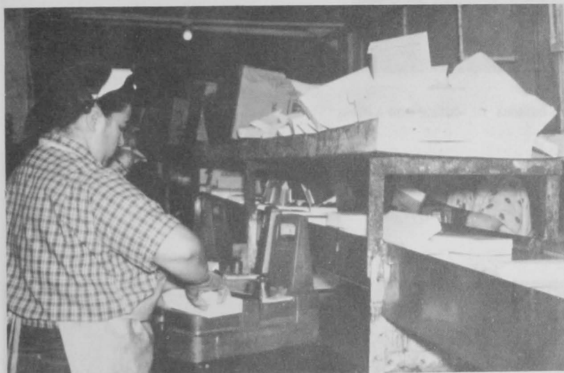
Figure 15.--A packer is using an "over-under" scale to check the weight of 1½-pound boxes.
