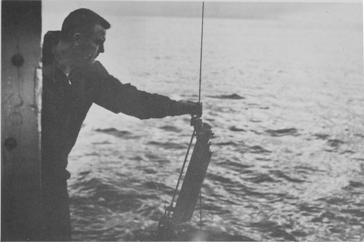
A Bureau oceanographer removes a reversing thermometer aboard the oceanographic research vessel, the Murre II .
