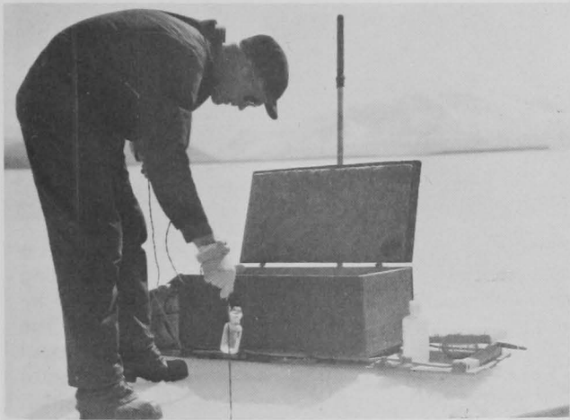
In studying limnology in a sockeye salmon nursery lake, a biologist prepares sample bottles inoculated with carbon 14. Uptake of radioactive carbon by microscopic plants in the water sample can be measured to determine the production rate of algae, the basic food for all aquatic life.
