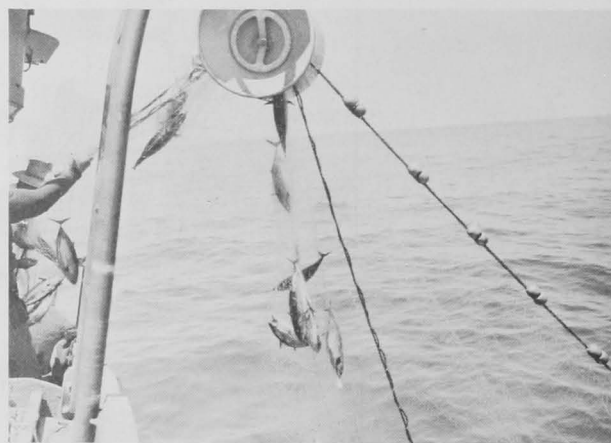
Figure 9.--Hauling in net with skipjack catch over the powerblock.
