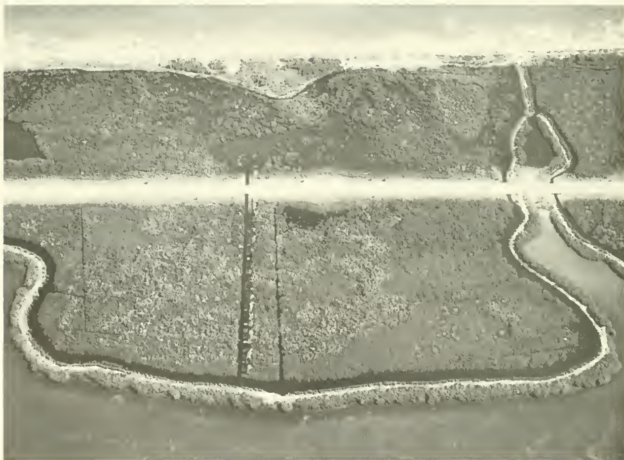
Type of impoundment developed by the Florida State Board of Health, under Bureau contract, that shows promise of controlling mosquitoes and serving the main needs of wintering waterfowl. (Photo by Florida State Board of Health)
