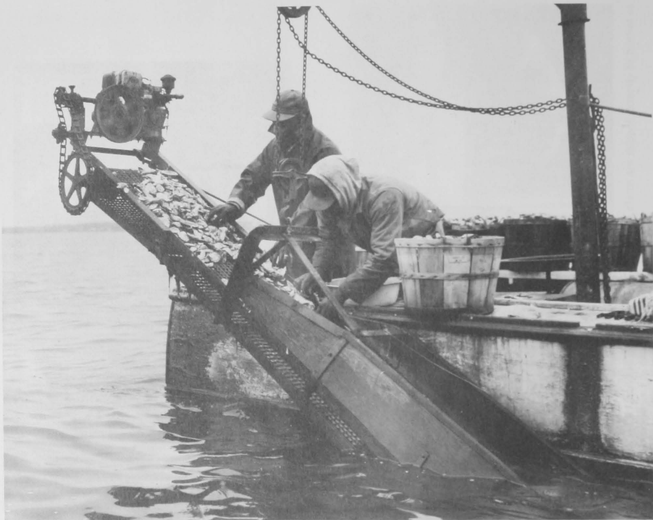
Figure 12.--Boat crew removes clams from the chain escalator belt. The small air-cooled motor (upper left) provides power for the belt.
