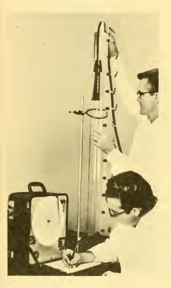
Determining salinity gradient with conductivity meter.
