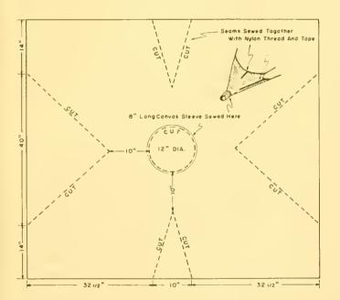
Pattern for cutting mesh body of beam net.
