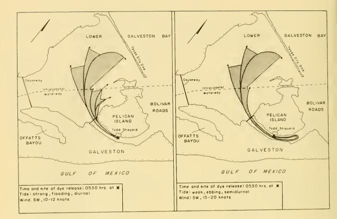
The distribution of rhodamine B dye in Galveston Bay ship channel on May 7, 1962 (left), and May 15, 1962 (right).
