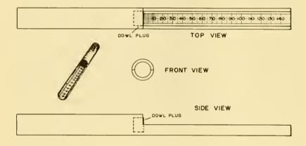
Shrimp measuring device made of plastic tubing.
