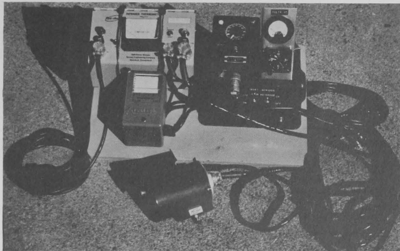
Photo at left:--Airborne infrared thermometer and accessory equipment; lower front, infrared optical detector head; upper left, infrared electronic circuitry and temperature indicator; below, strip chart recorder; upper right, intervalometer for visual readout timing, clock and voltmeter.
