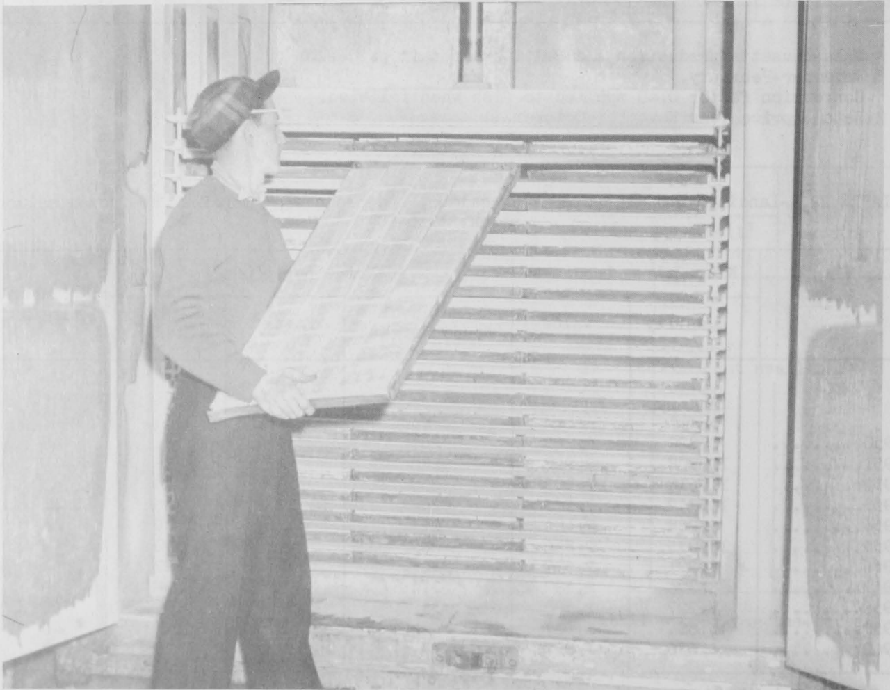
Figure 10.--Preparation of fishery products for marketing requires the use of specialized equipment. Shown here is a plate-type quick freezer used by a New Bedford firm for freezing consumer-packaged scallop meats.
