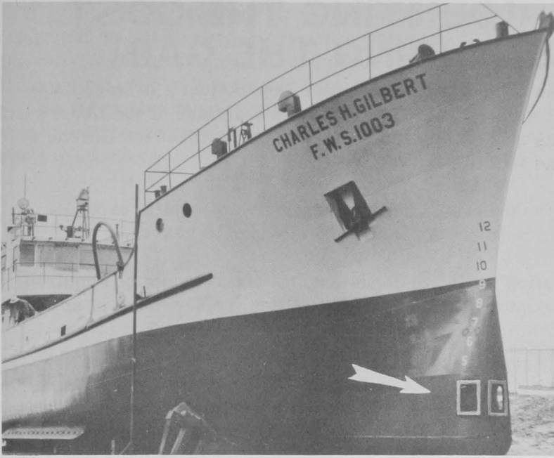
The Bureau's M/V Charles H. Gilbert has been modified for direct observation of fish from viewing chambers fore and aft. Use of a small, specially-designed submarine, which would be more effective, is being studied.
