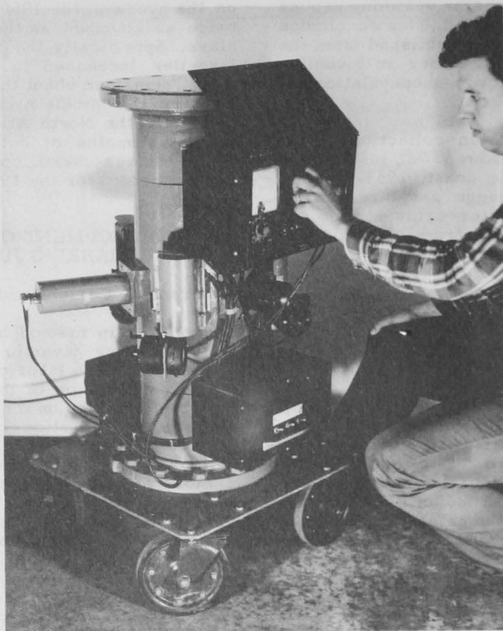
An experimental electronic detector for menhaden marked with fluorescent pigments.
