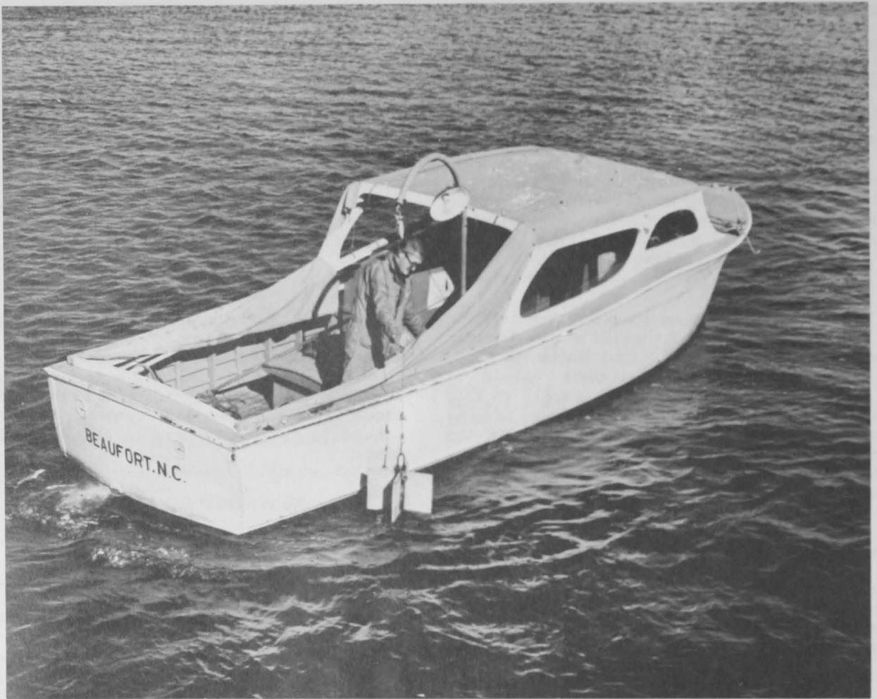
Using confined submerged drag to estimate current velocity in Newport River estuary, N. C.
