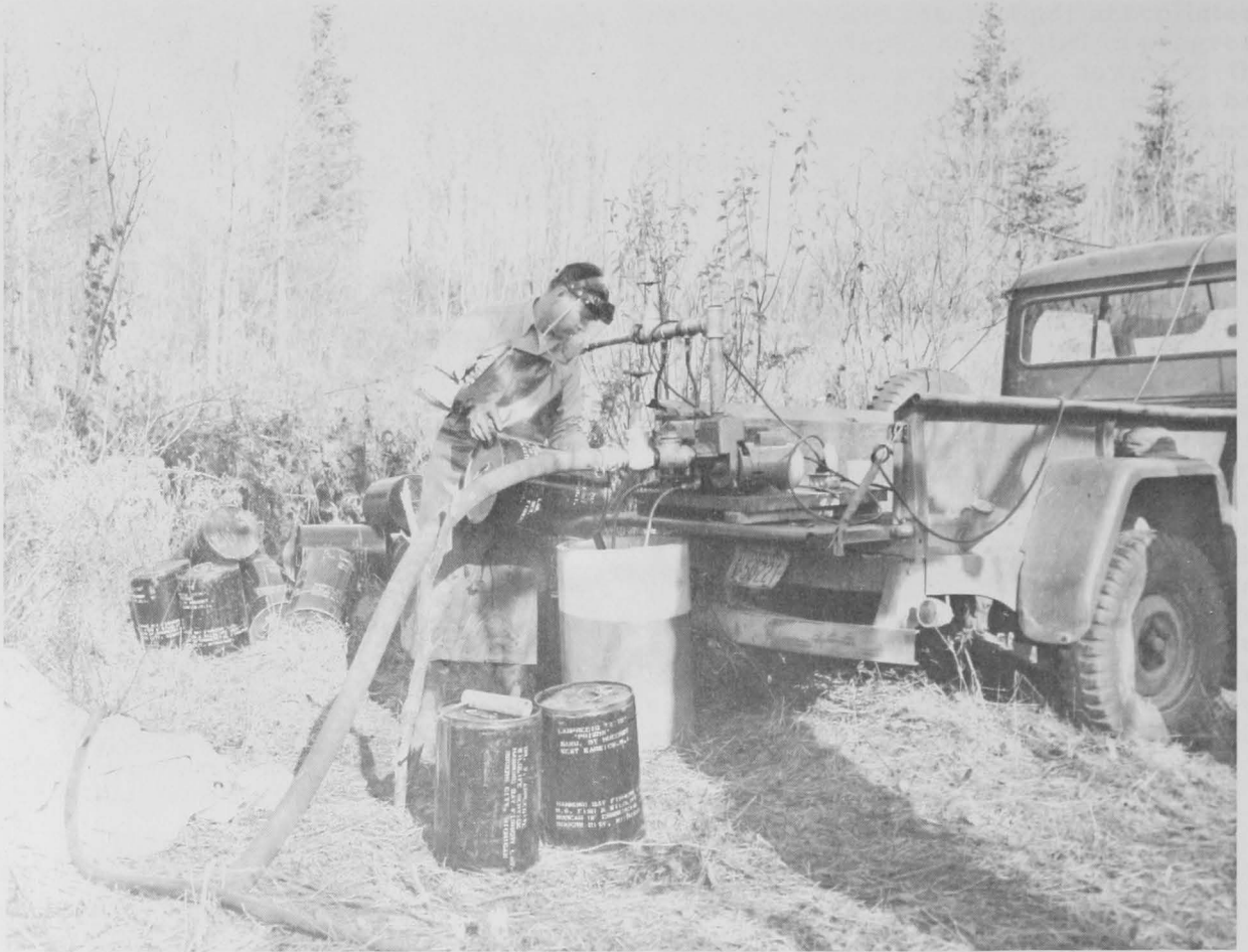
Feeder mechanism that maintains critical level of selective toxicants in streams that will destroy sea lamprey larvae and not harm fish.
