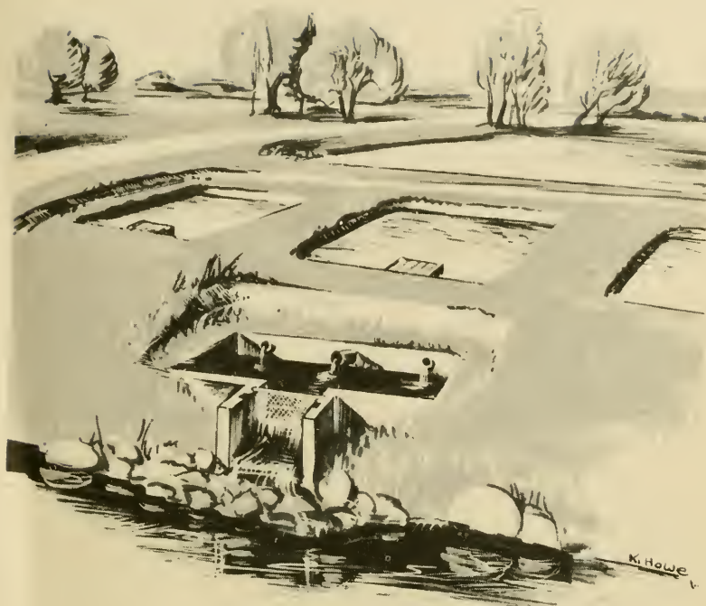
Figure 9.—Collecting basin constructed outside the ponds.
