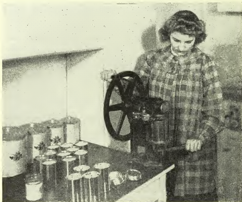
Figure 3.—Typical can-closing machine adapted to the home canning of fishery products.
