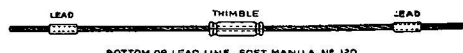
BOTTOM OR LEAD LINE. SOFT MANILA NO 120 LEADs ARE 8' LONG, MADE OF SHEET OF LEAD BEATEN TIGHT ON LINE THIMBLE TURNED IN TWO PIECEs TO FIT ROPE AND LASHED ON
