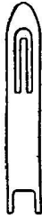
NET MAKER'S NEEDLE; MADE ALL SIZES FROM 3" OR 4" UP TO 2'; GENERALLY OF HARDWOOD, BUT SOMETIMES OF BRASS OR OTHER MATERIAL
