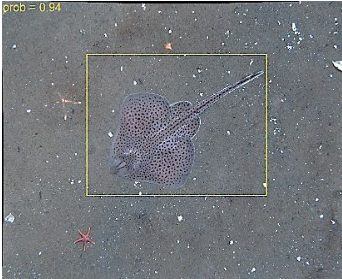
Figure 4-5. Imagery from the HabCam survey operations with an example of skate detections using VIAME/YOLO v2.
