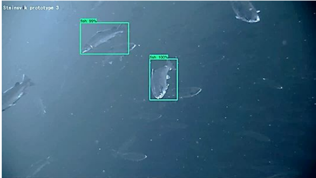
Figure 2-13. NORCE has used machine learning for automatic fish detection, lice counting, and prediction of fish growth and health of farmed salmon.
