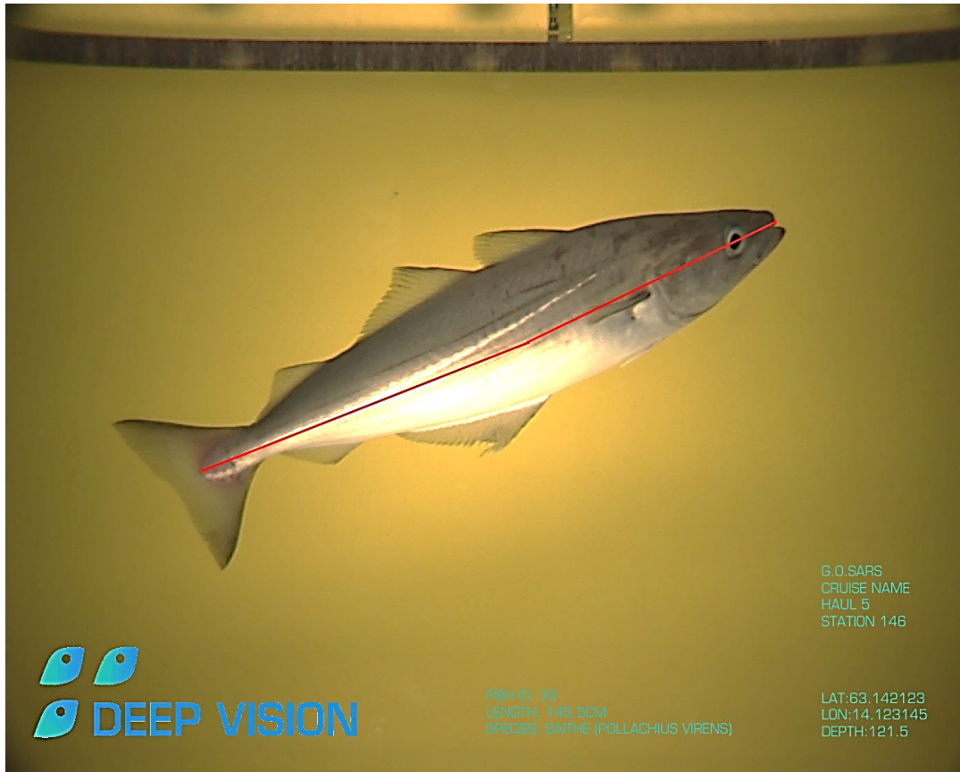
Figure. 3-2. Image of fish and fish length measures from the Deep Vision system.
