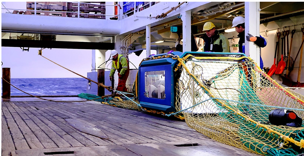
Figure 3-4. Deployment of the Scantrol Deep Vision stereo camera system.
