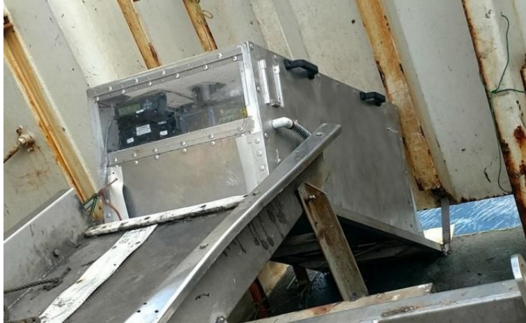
Figure 5-1. Camera chute system deployed on a Bering Sea trawler.
