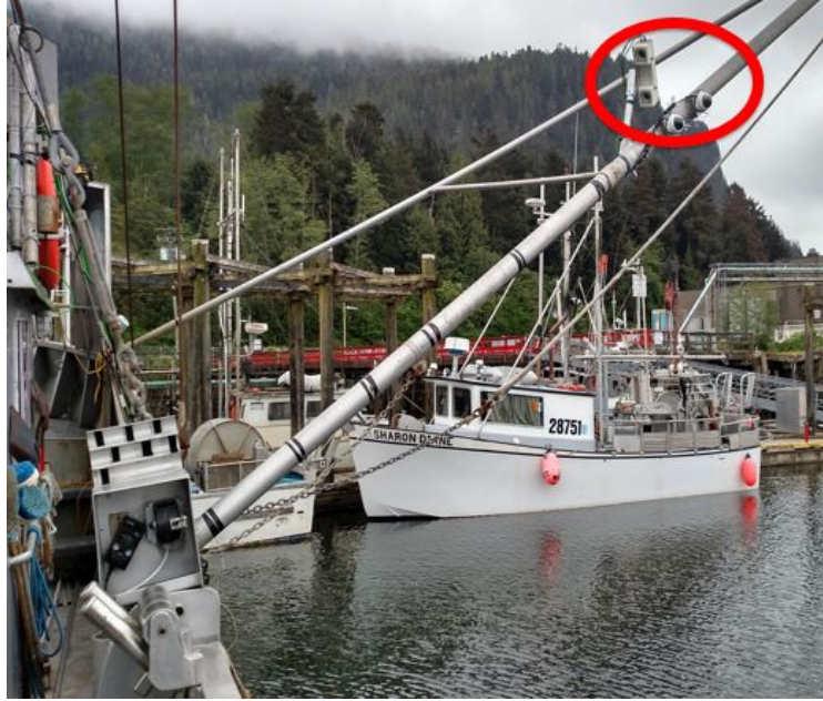
Figure 5-3. Stereo camera placement (vertical camera system) on an Alaskan longline vessel.
