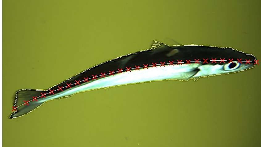
Figure 3-6. Result of the automatic fish segmentation and measurement pipeline. The specimen is segmented analyzing the image to background saturation ratio. The measurement is later on performed by computing a third order polynomial using RANSAC approximating the shape of the fish-blob skeleton morphological operation. The length of the fish has been estimated as 267 mm.
