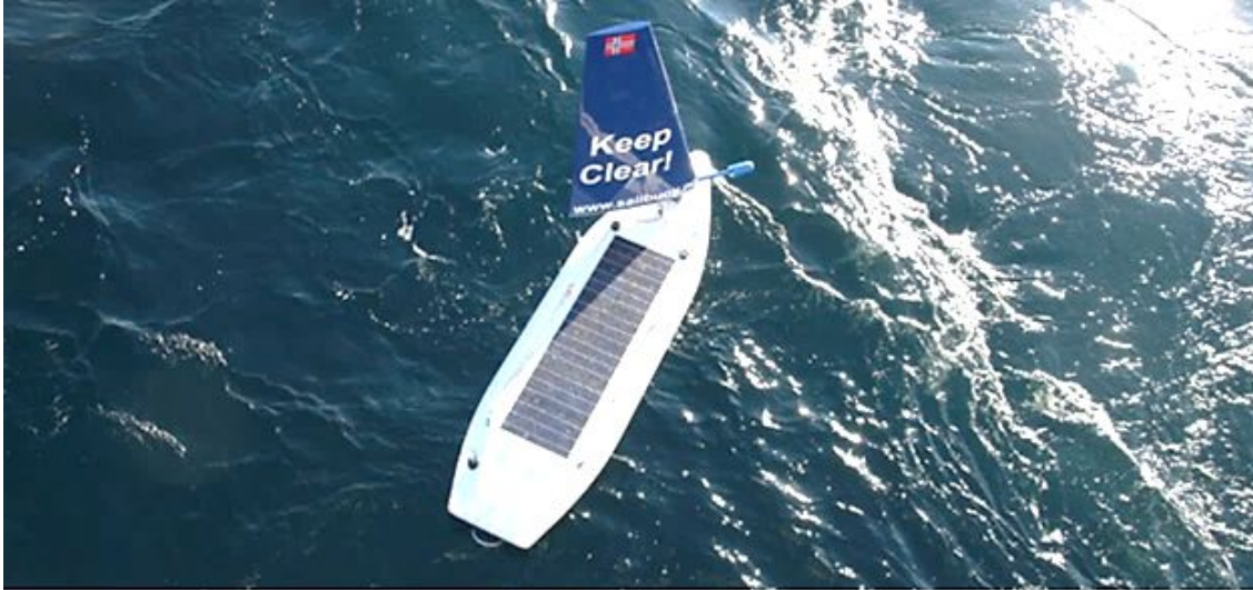
Figure 2-11. The Sail Buoy is the first unmanned surface vehicle that completed an Atlantic crossing.
