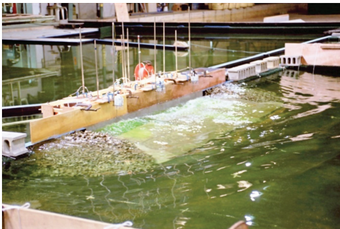
Figure 5. Photograph of seawater exchange structures with blockwork mounds in the experiment.
