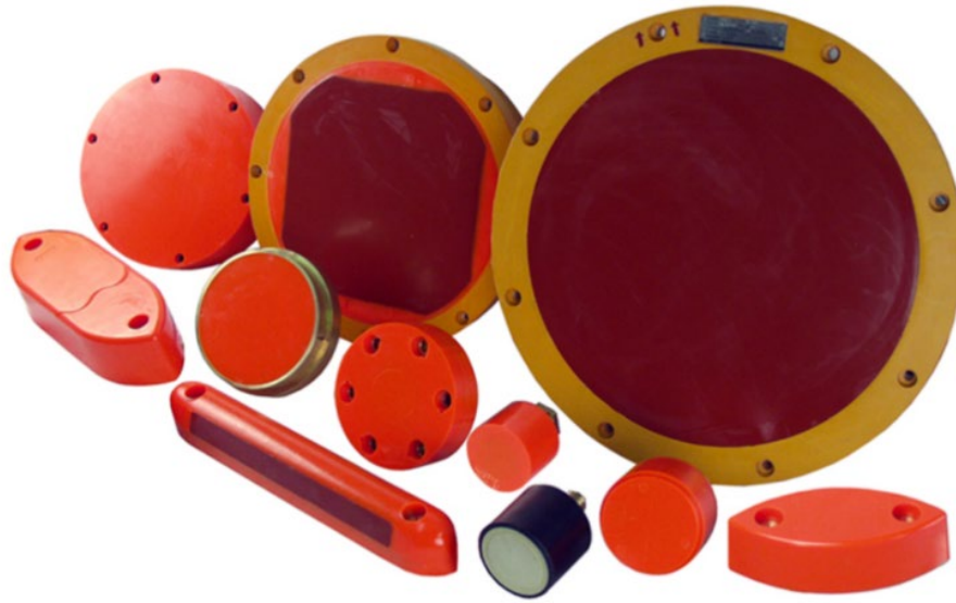
Figure 6-1. Transducers come in different sizes and shapes depending on frequency and beam width. For the same beam width, transducers become smaller as frequency increases and wider beam transducers are physically smaller. Most transducers generate circular acoustic beams, but some generate elliptical beams. Mind that lower frequency transducers are not suited for portable use due to size and weight. The largest transducer in the picture (top right) is 18 kHz, has a diameter of 63 cm and weighs 85 kg.
