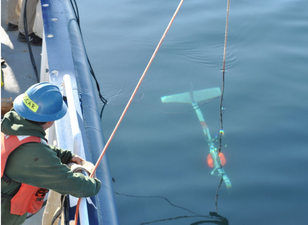
Figure 4-5. A simple towbody towed from the side of a research ship. The simple frame holds a single transducer. The rear tail stabilizes the towbody while underway.
