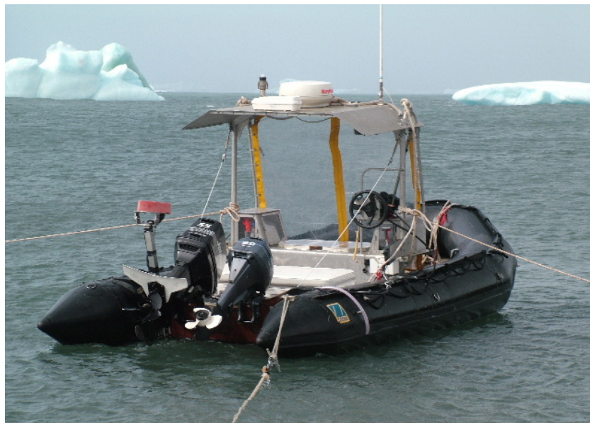
Figure 4-4. A transom-mounted retractable pole with 120-kHz split-beam transducer (Simrad ES120-7F). For deployment, the pole is lowered into the water and locked with a pin such that the transducer is deeper than the propeller, to reduce bubble noise, and project downward.
