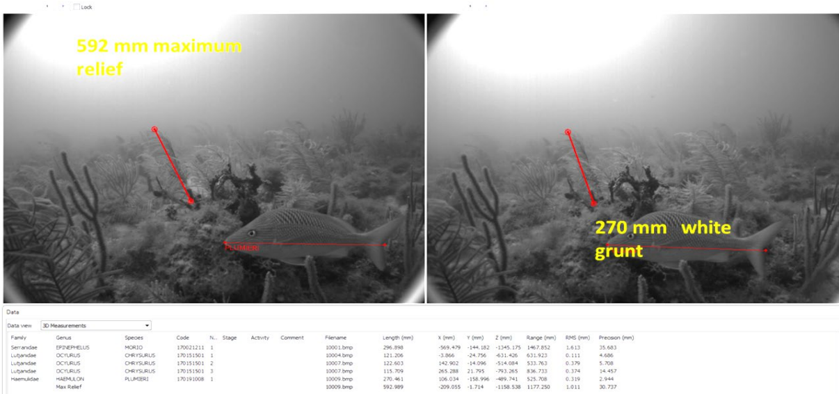
Figure 5-3. Example of stereo image of a white grunt. Calibrated stereo images allow for measurements of fish size composition but also descriptions of the reef relief and other habitat metrics.
