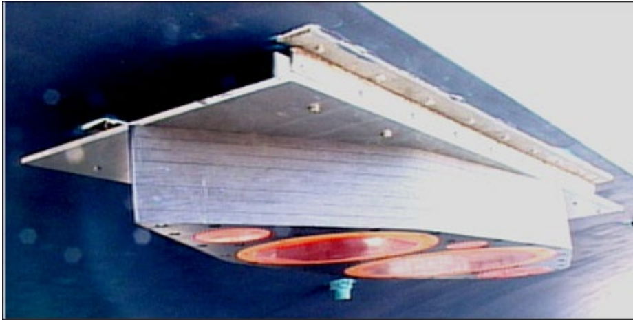
Figure 4-1. A hull-mounted five-frequency transducer array (far to near: Simrad ES70-7C, ES18-11, ES200-7C, ES38B, ES120-7C). The array is temporarily attached to the hull using angle steel that is bolted through the fiberglass. The cables are routed through a standpipe with a 3" diameter ball valve to the echosounder transceivers. The laminated HDPE fairing redirects bubbles away from the transducers.
