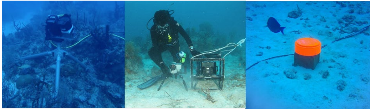
Figure 10-1. Example of a stationary deployment for imaging sonars (left panel showing DIDSON and Kongsberg M3), a diver deploying an imaging sonar and video camera (middle panel), and an upward facing split-beam echosounder (right panel) deployed near Aquarius Reef Base in the Florida Keys.
