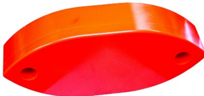
Figure 6-2. The Simrad ES38-18/200-18 omni-transducer combines the 38 kHz and 200 kHz frequencies which can be utilized to improve target discrimination and identification. Due to the relatively wide beam width (18° at both frequencies) the transducer is small (416x172x94 mm) and with a weight of 7.3 kg, it is suitable for portable use. The boat shape is chosen for good hydrodynamic performance.
