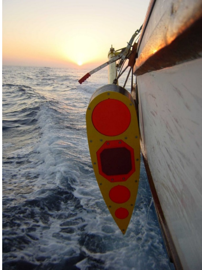
Figure 4-3. A portable four-frequency transducer array (top-bottom: Simrad ES70-7C, ES38-12, ES120-7C, and ES200-7C). To deploy, the array is lowered into the water such that the transducers are > 1-m deep and projecting downward, and stabilizing lines are ratcheted tightly, fore and aft.
