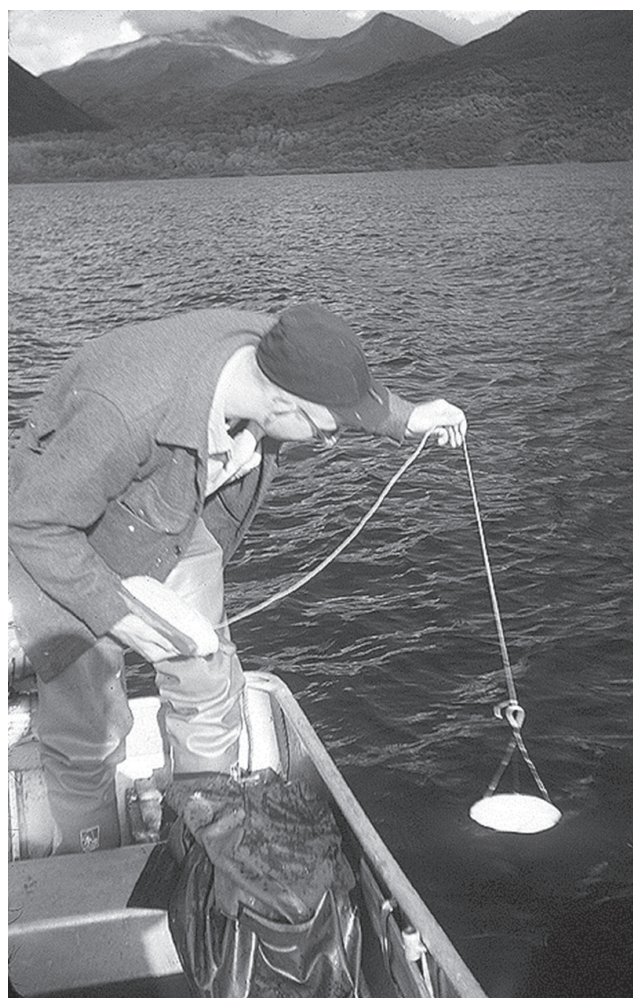
Fisheries Research Institute biologist Bill Mulligan measuring water transparency with a Secchi disk, Karluk Lake, 1952. (Charles E. Walker, Sechelt, BC)
