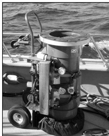
Figure 4. Hyperbaric chamber set on end prior to fish insertion.
