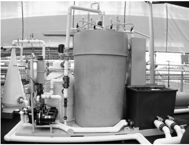
Figure 2. Example of a recirculating water treatment system.
