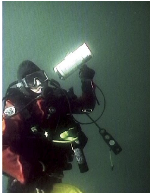
Figure 3. A diver holding a Datasonics DPL-275-H dive receiver. Scuba observations are made at least weekly to monitor crab movements.
