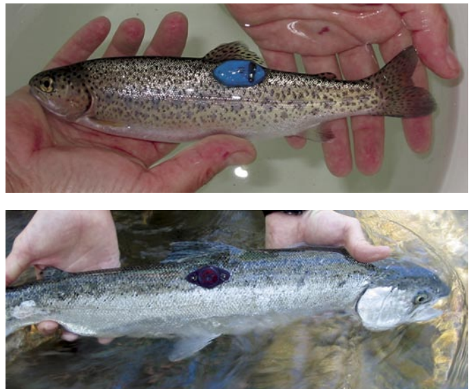
Figure 2. External attachment of iBKrill tag on steelhead smolt (upper) and the larger iBCod tag on steelhead (lower).
