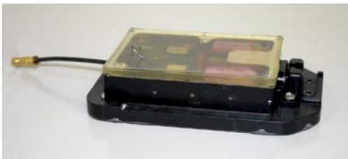
Figure 1. A prototype remote release platform that is being developed by Advanced Telemetry Systems.
