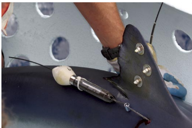
Figure 3. The anchoring hardware used to attach the PAT and SPOT tags to the sharks.
