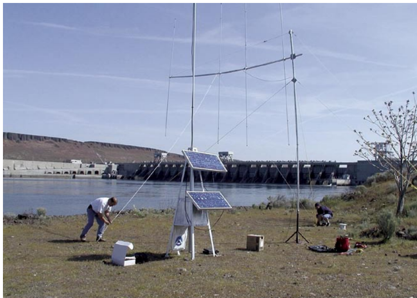
Figure 1. A typical stationary radiotelemetry site, near McNary Dam on the Columbia River. An antenna and two solar panels provide power to the radiotelemetry receiver located in the cabinet under the bottom solar panel.
