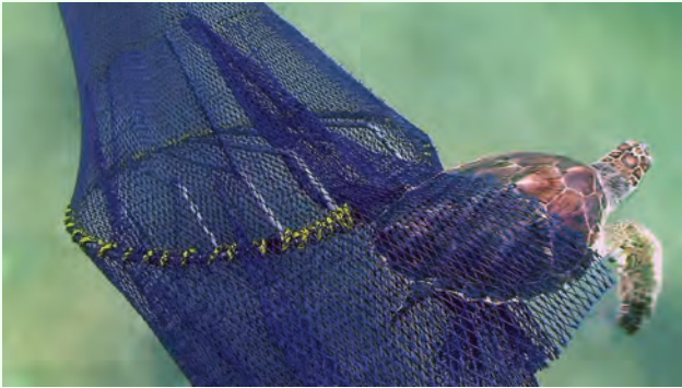
A loggerhead sea turtle escapes from a net equipped with a turtle excluder device (TED).
