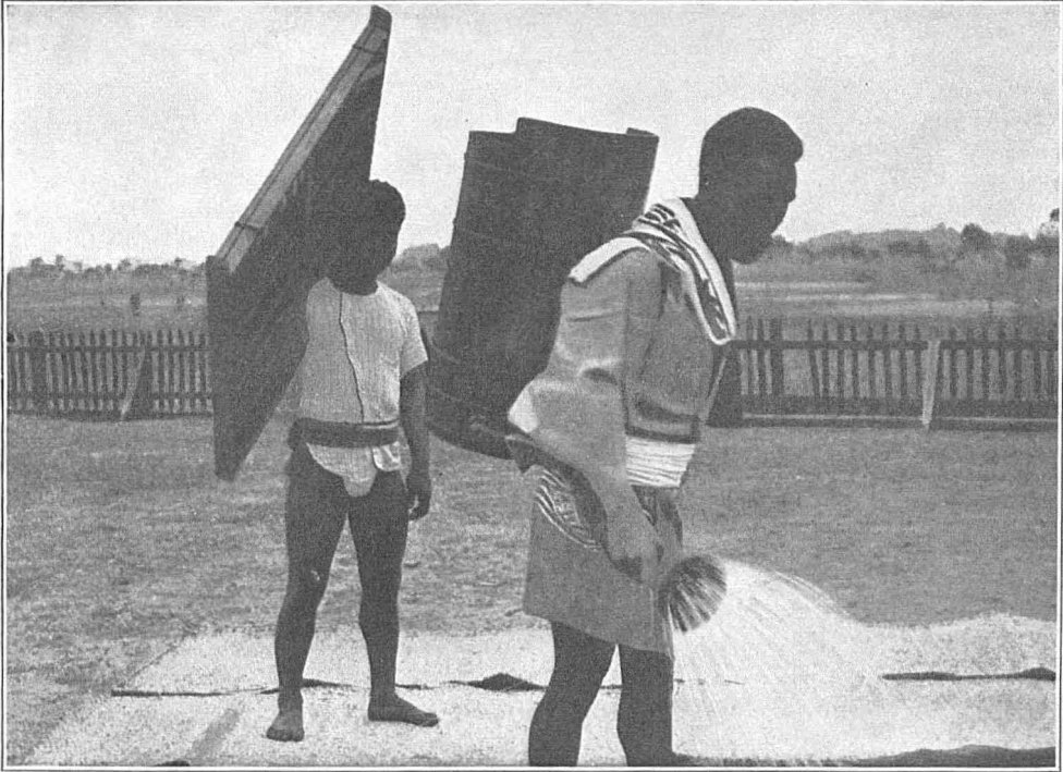
SPRINKLING THE SHEETS TO PREVENT CURLING.
