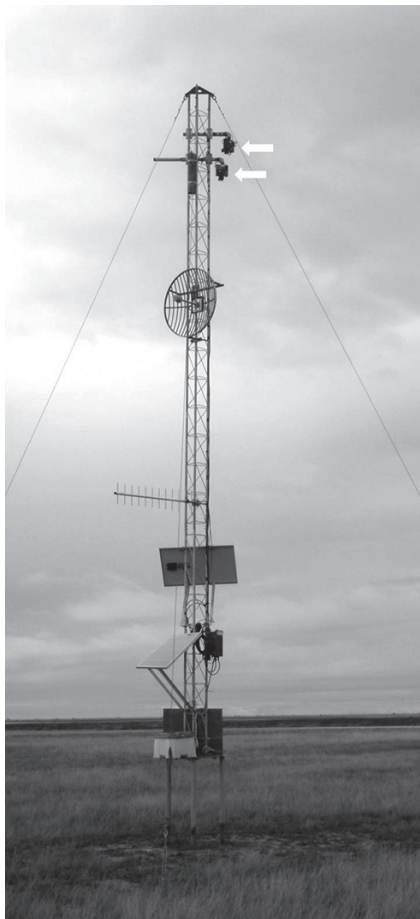
Figure 2.—Tower and mounted cameras used to monitor Cook Inlet beluga whales in the Little Susitna River. Arrows indicated the location of the two cameras mounted near the top of the tower.
