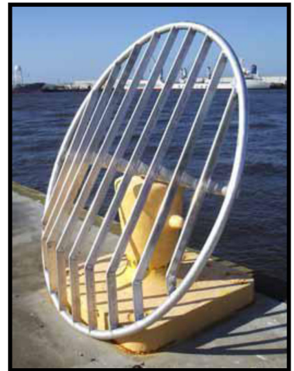
Figure 20.—Flat Bar TED leaning against a mooring. (Source: J. Watson. 2005. Sea Turtle Bycatch Reduction Research in the U.S. 1st Annual Meeting of the Bycatch Reduction Consortium, 1–2 June 2005, Boston, Ma. http://www.neaq.org/documents/conservation_and_research/bycatch_consortium/2005_meeting/john_watson.pdf ).
