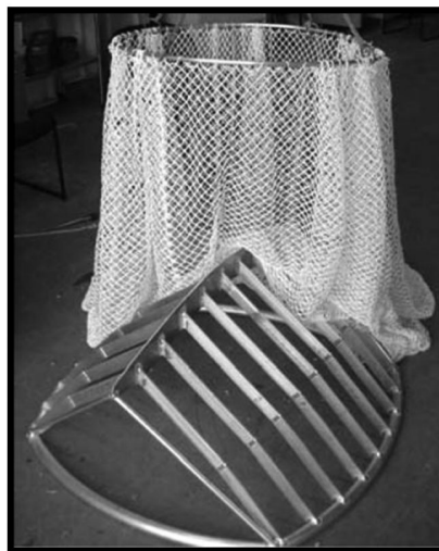
Figure 21.—The Double Shot TED frame prior to installation in webbing extension tube (Source: USDOC, 2011).
